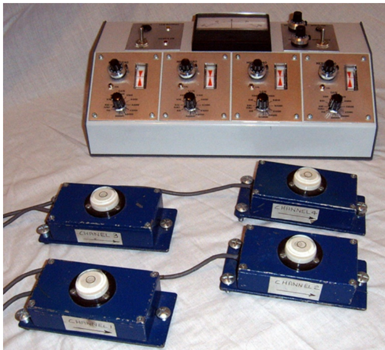
Figure 1 - Prototype four channel tower movement measurement electronics being developed in about 2005 – (Photo from CCCBR Towers and Belfries Committee Records)
