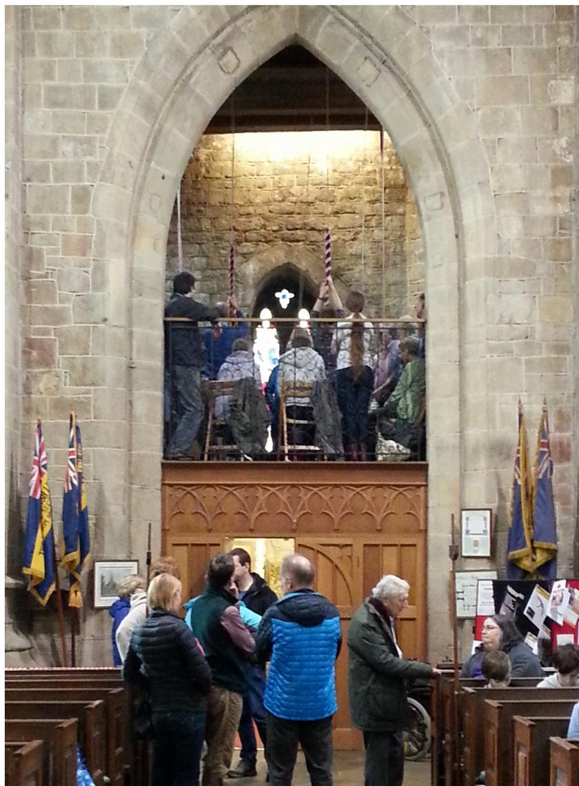
*Open gallery style ringing room. This design offers useful enclosed space at ground level. (The addition of a glass screen or long openable curtains across the arch would enable the ringing room to be heated when necessary.)*
